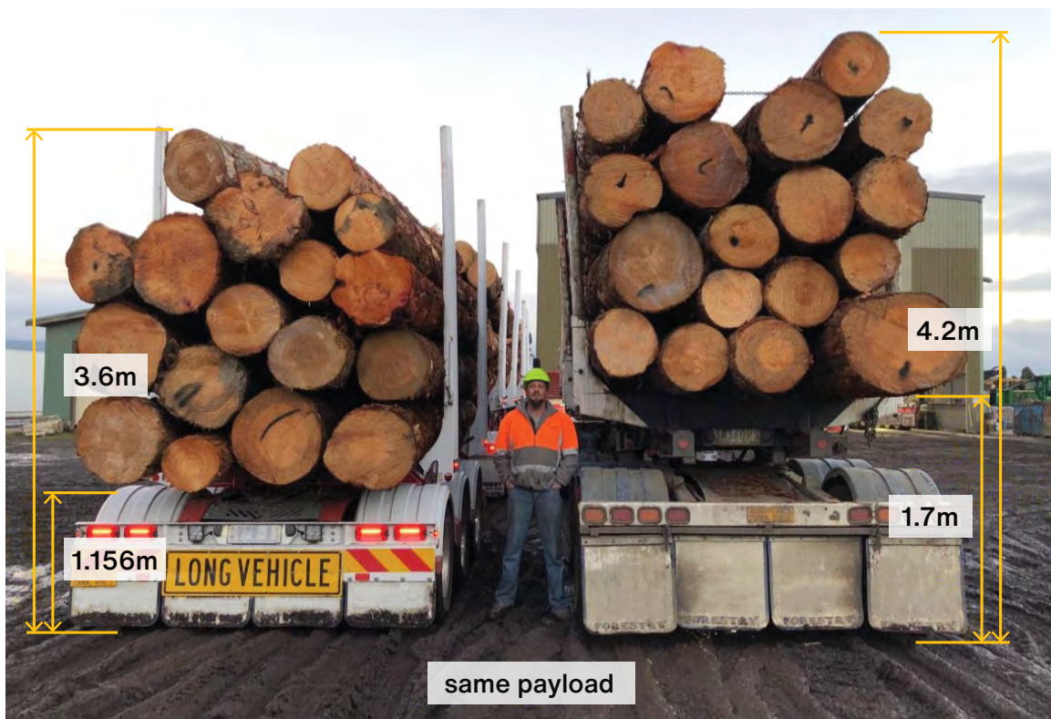
Figure 7.2. Step deck trailer with 19.5" wheels and low bolsters compared with flat deck with 22.5" wheels and high bolsters.
