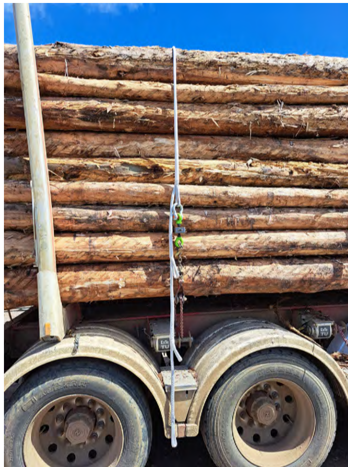
Figure A.3. A length of UHMWPE rope with eye splices at different lengths was used to position this load cell correctly. (Refer Testing lashing tension)
