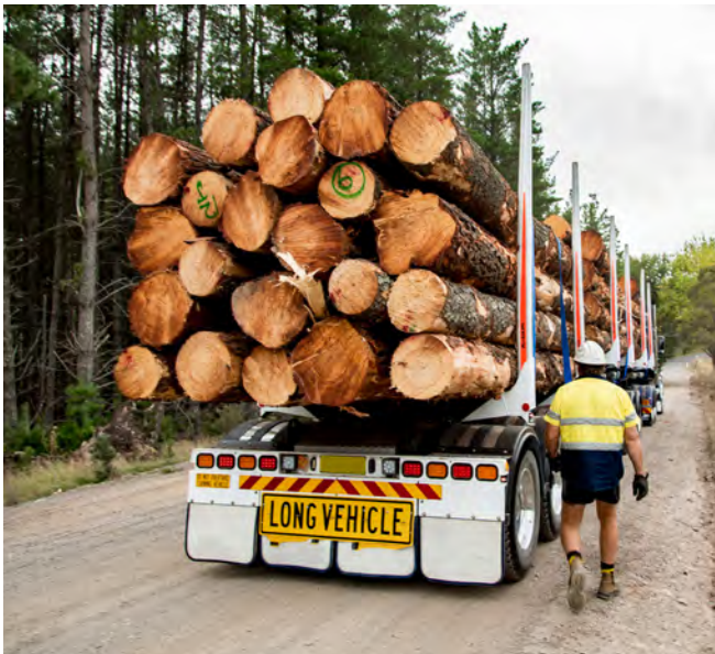
Figure 12.6. A well-constructed load with a suitable crown improves restraint effectiveness
