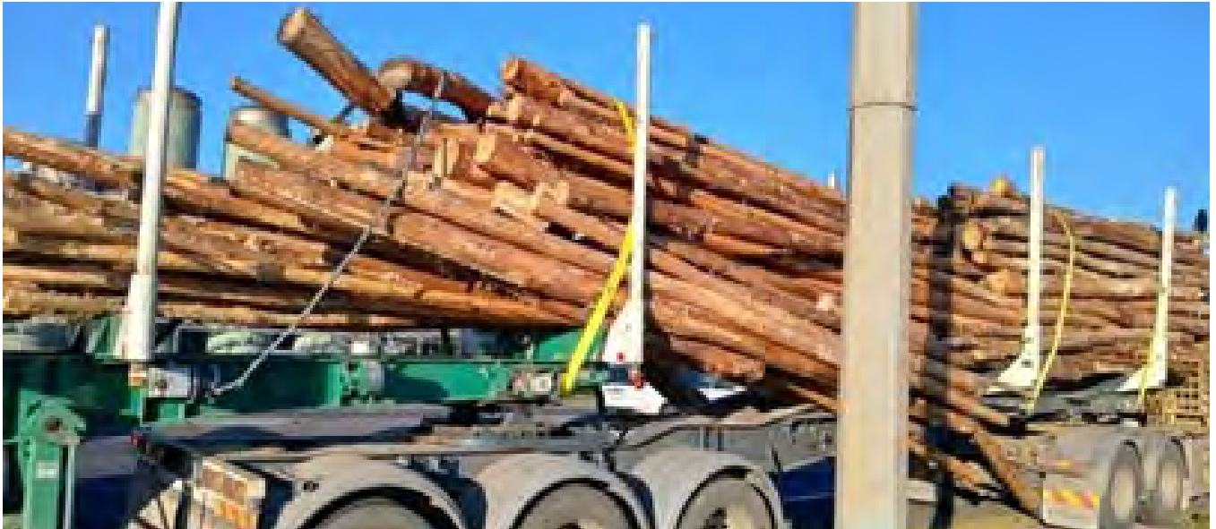
Figure 7.5. Without a headboard on the rear trailer, logs were not blocked (Refer to 7.5.2)
